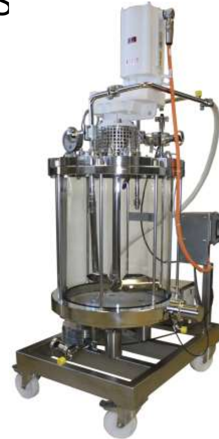
InPlace D596 column in Belgium Used in agitated mode
